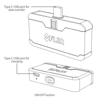
⚠ Do not interchange USB type C ports for charging and data transfer.
